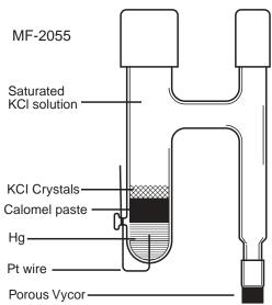
**CAUTION:** Mercury and calomel are POISONOUS substances. They should be handled carefully, and waste material should be disposed of in accordance with accepted procedures. If the calomel vial has broken in shipping, DO NOT OPEN the protective outer plastic enclosures. Dispose of the vial and contents as a single unit. Call BAS (1-800-845-4246) for a replacement.
