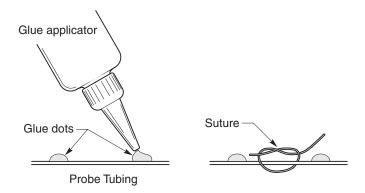
Do not tie the sutures so tightly around the probe tubing that flow is cut off or restricted.
