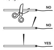
Connect the other end of the probe to a syringe pump using flanged tubing connectors (see 13 below). Begin perfusion at 1 or 2  $\mu$ l/min. Allow several minutes for flow to be established through the probe. If flow does not occur, cut away an additional 5-6 mm of probe tubing. Recheck until flow is established. Turn off the pump or disconnect the probe before proceeding.
